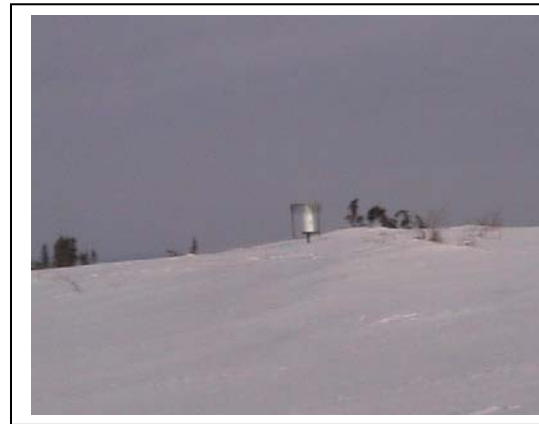
This moisture gauge is located at the Yukon border and collects both snow and rainfall.
